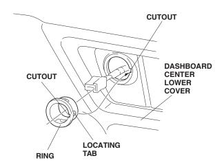
8. Connect the vehicle 2-pin connector to the new socket.
