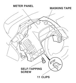
Apply masking tape to the instrument panel as shown, and remove the center panel (two bolts, 10 retaining clips, and unplug the vehicle connectors).
