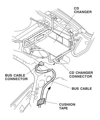
38. Fold the excess BUS cable, and secure the BUS cable to the holes in the rear seat panel with the two wire ties with clip.
