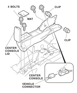
13. Remove the center console (four bolts, two clips, and the vehicle connector).
