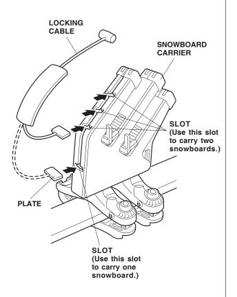
15. After loading each snowboard on to the carrier, adjust it with the help of the board supports so that the top edges are level and the boards are as far down in the carrier as possible. To secure the snowboard, use the key to open the covers, then insert the locking cable stoppers into the holes of the carrier covers.
