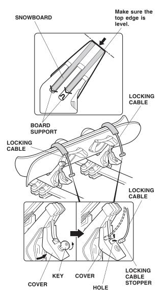
16. Check that the locking cables are installed securely, then close the covers.
