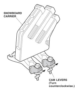
5. Attach the two bottom clamps to the two top clamps.
