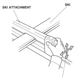
Rock the ski attachment in all directions to make sure it is installed securely.
