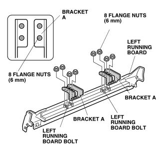
17. Position the left running board on the vehicle, and secure brackets A using four flange bolts. Make sure the inner fender fits on the inside of the left running board end cap. Align the clips installed in step 15 to the holes in the body panel, and push them into position.
