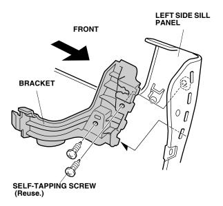
13. Install the bracket to the left running board with one of the screws removed in the above step.
