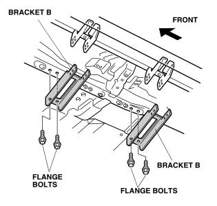
19. Secure brackets A and B using eight flange bolts and eight 8 mm flange nuts.
