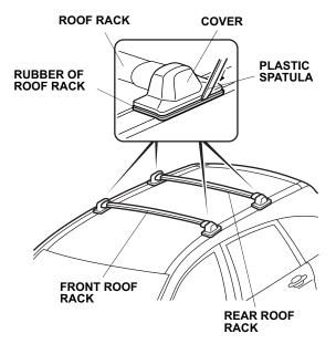
7. After installing the roof rack, rock each rack to make sure it is secure.
