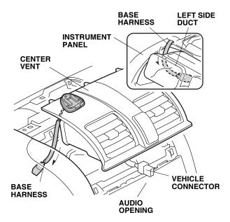
36. At the meter opening, plug the navi harness 2-pin connector into the base harness 2-pin connector. Secure the 2-pin connectors to the vehicle harness with one wire tie.
