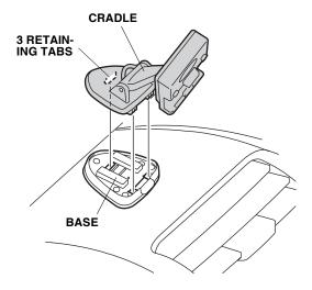
38. Open the antenna of the navi unit, and fit the bottom of the navigation unit into the cradle (terminal and one retaining tab). Tilt back and snap into place.
