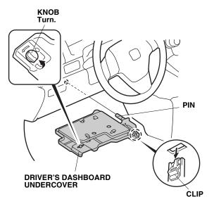
10. Remove the driver's dashboard lower cover (seven clips).
