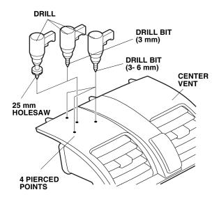
28. While wearing eye protection, drill the center hole to 25 mm. First drill with a 3 mm drill bit, and then finish with a 25 mm holesaw. Remove any burrs. Only enlarge the center hole to 25 mm.
