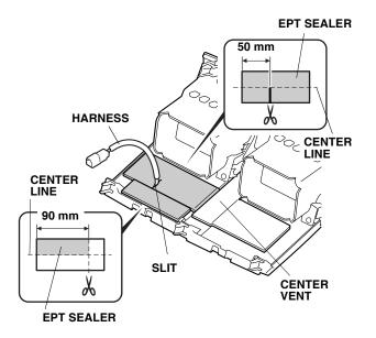
34. Using scissors, cut one EPT sealer in half, then cut a 90 mm piece from one of the halves. Attach the 90 mm piece of EPT sealer to the center vent in the area shown.
