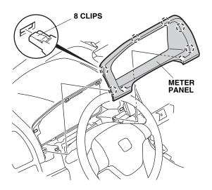
8. Remove the meter panel by removing the three self-tapping screws. Slide the meter to the left and disconnect the two vehicle connectors. Keep the meter in the upright position.
