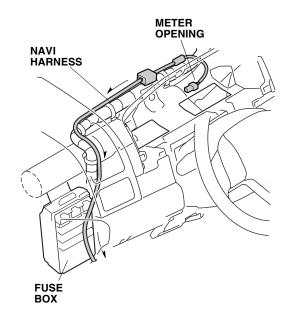
Plug the navi harness 6-pin connector into the fuse box.
