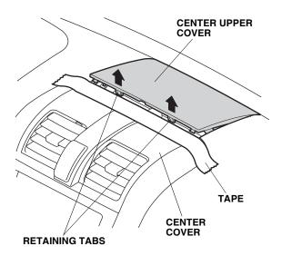
4. Using a flat-tip screwdriver, release the two retaining tabs from the center upper cover.
