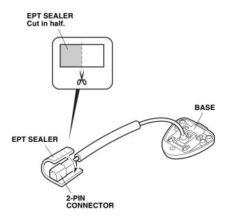
30. Route the 2-pin connector from the base through the rubber seal and into the 25 mm hole in the center vent. Note the direction of the rubber.
