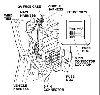
Secure the navi harness to the vehicle harness with two wire ties.
