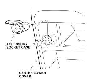
7. Slide the ring into the hole in the center lower cover in the direction shown.
