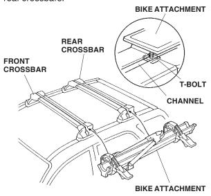
7. Turn and adjust the mounting lever to lock the bike attachment to the roof rack. Check for firm pressure while you push down on the mounting lever to lock it into place.
