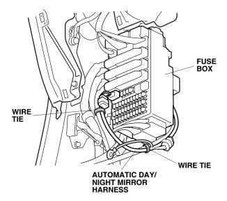
25. Remove the vehicle bolt from the fuel lid opener. Attach the automatic day/night mirror harness ground terminal with the ground bolt supplied.
