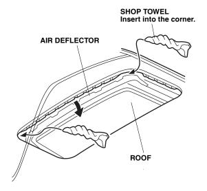
4. At the right front corner of the moonroof opening, mark with a felt-tip pen along the rise from the flange end of the opening approximately 40 mm as shown.
