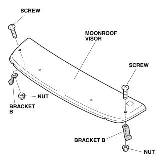
12. Align the moonroof visor on the install location and align brackets B on the center of the protective tape and install temporarily. Do not tighten the two screws and two nuts yet.
