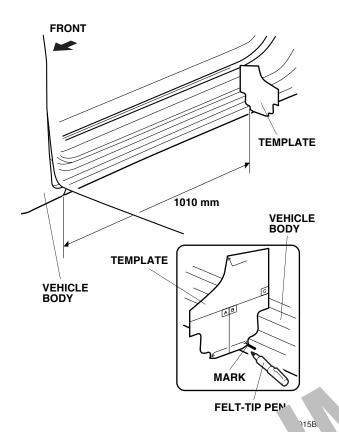
4. Position the template (C) on the vehicle body. Using a felt-tip pen, mark the vehicle body at the distance shown.
