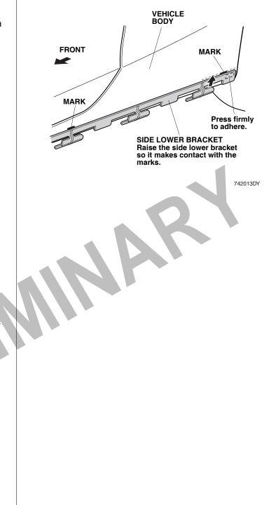
10. Press the front end of the side lower bracket (where you removed the adhesive backing) to adhere the part firmly to the vehicle body.
