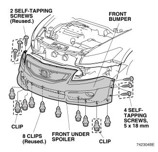
32. While applying pressure to the front under spoiler, carefully remove the adhesive backings from the center outwards. After removing the backings, hold the front under spoiler firmly against the front bumper with the palm of your hand for 30 seconds.
