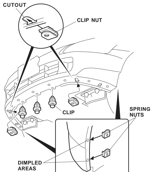
2. Slide the two spring nuts over the dimpled areas of the front bumper on each side.
