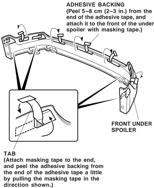
6. Position the front under spoiler on the front bumper, and temporarily install the four fender bolts, three stepped bolts, five flange nuts, and four self-tapping screws. Check that the molding on the front under spoiler is not tucked under the front under spoiler.
