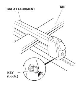
5. With the ski attached, rock the attachment in all directions to make sure it is installed securely. Adjust as necessary.
