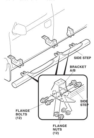
9. Adjust the location of the left side step so that even clearance is obtained between the side step and body, then tighten the flange bolts you installed in step 7. Torque 10 flange bolts to 27 N·m (20 lbf·ft), and the one remaining flange bolt to 7 N·m (5 lbf·ft) as shown.
