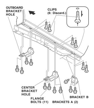
Install the two brackets A and one bracket B to the body using 11 flange bolts. Thread the flange bolts in about 3 to 4 threads. When installing brackets A, use the outboard bracket holes for the front bracket, and the center bracket holes for the center and rear brackets. 8. Position the side step to the brackets using the 12 flange bolts and 12 flange nuts. Thread the flange bolts in about 3 to 4 threads.
