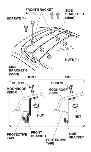
8. While holding the visor in place, install the four screws, four nuts, and four brackets A and B with the end of each bracket hooked to the lip of the moonroof opening. Do not tighten the screws yet.
