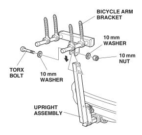
3. Install the torx bolt with two 10 mm washers and the 10 mm nuts. Tighten the torx bolt securely.
