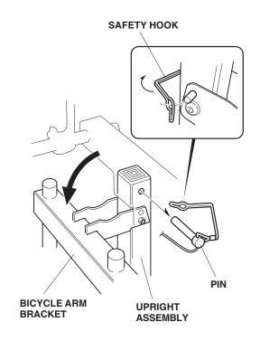
2. Reinstall the pin and safety hook.
