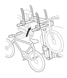
3. Tighten the bicycle arm straps securely around the bicycle frame.
