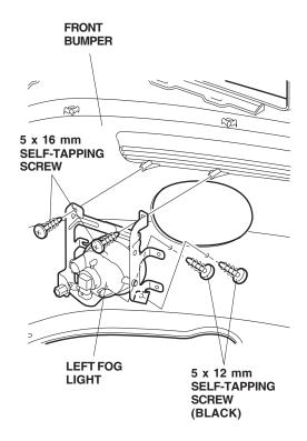
11. Attach the left trim to the front bumper with three  $5 \times 16$  mm self-tapping screws.
