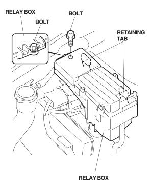
15. Release the four retaining tabs, and remove the under-hood fuse/relay box upper cover.
