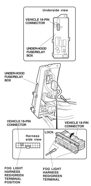
21. Reconnect the vehicle 18-pin connector into the under-hood fuse/relay box.
