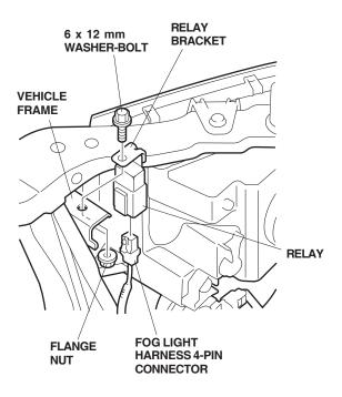
33. Plug the fog light harness 4-pin connector into the relay.
