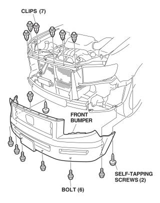
4. On the inside of the front bumper, locate the fog light identification marks on the left side. Using a pushpin, mark the front bumper at each of the eight marks as shown.
