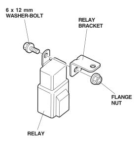
32. Attach the relay bracket to the vehicle frame with one 6 x 12 mm washer-bolt and one flange nut.
