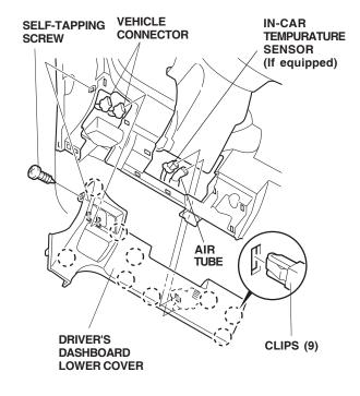
41. Remove the switch lid from the driver's dashboard lower cover, and install the fog light switch into the driver's dashboard lower cover.
