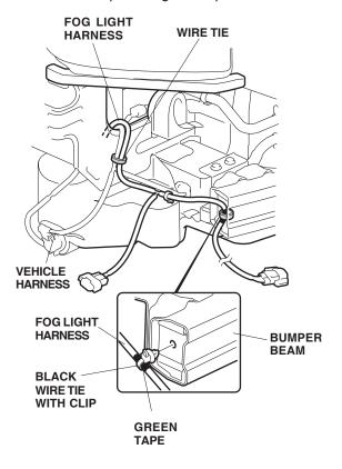
36. Secure the fog light harness to the bumper beam:
