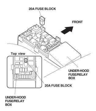
28. Attach the 20A fuse label onto the inside of the under-hood fuse/relay box upper cover.
