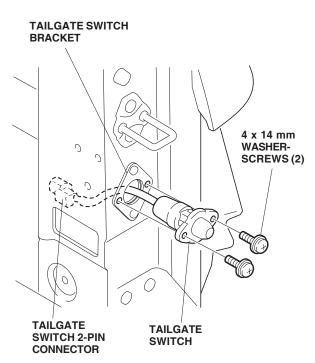
66. Plug the backup sensor harness 2-pin connector into the tailgate switch 2-pin connector.
