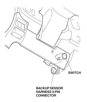
89. Using isopropyl alcohol on a shop towel, clean the areas where the EPT sealer will attach. Attach the EPT sealer to the driver's console side trim in the area shown.
