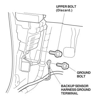
79. Route the backup sensor harness up and along the vehicle frame, and secure it to the vehicle harness and frame with five wire ties.
