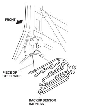
48. Pull the 2-pin connector up along the vehicle panel, and into the cargo area. Seat the backup sensor harness grommet into the body hole.
