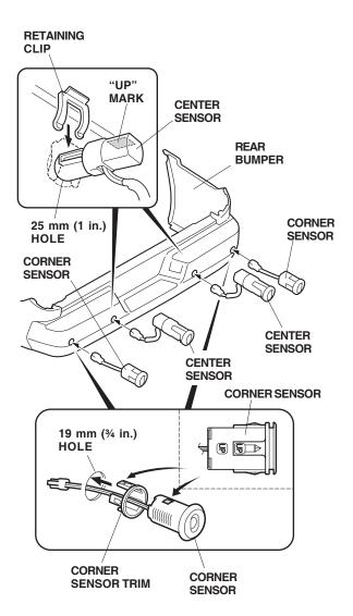
41. Slide the two center sensors into the 25 mm (1 in.) holes with the "UP" mark facing up. Secure the center sensors with one retaining clip for each sensor.
