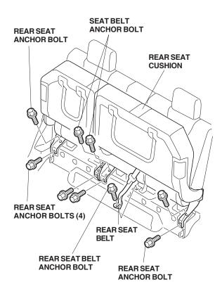
16. Remove the eight rear seat anchor bolts, and remove the rear seat cushion.
