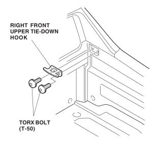
31. Remove the front bed panel (six torx bolts).
