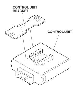
72. Plug the backup sensor harness 22-pin connector into the control unit, and insert the control unit bracket into the hole in the rear vehicle panel. Secure the control unit bracket with one flange bolt.
