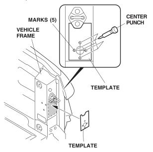
60. While wearing gloves and eye protection, unua 26 mm hole and four 8 mm holes through each of the marked locations. First drill with a 3 mm drill bit, then finish the center hole with a 26 mm hole saw and the outer holes with an 8 mm drill bit.
