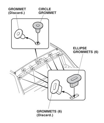
27. On the inside of the rear roof trim, remove and discard the clips, and install the seven new clips to the rear roof trim.
