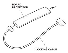
14. Insert the locking cable plate into the slit in the snowboard carrier. To carry one snowboard, insert the plate into the lowest slit. To carry two snowboards, use one of the upper three slits in the carrier.
