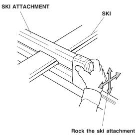
in all directions to make sure it is installed securely.
