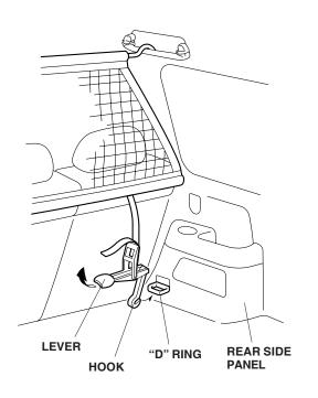
7. Adjust the length of the straps as needed. Lower the handle and snap the lever closed against the hook.
