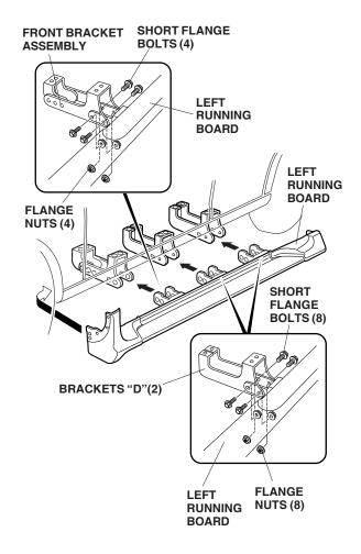
7. Insert the retaining tab on the left running board into the square hole in the left front inner fender. Position the left running board on the left front inner fender and install the five self-tapping screws that you removed in the step 2.
