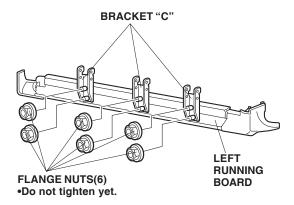
6. Position the left running board on the brackets using the twelve short flange bolts and twelve flange nuts. Thread the short flange bolts in about 3 or 4 threads.
