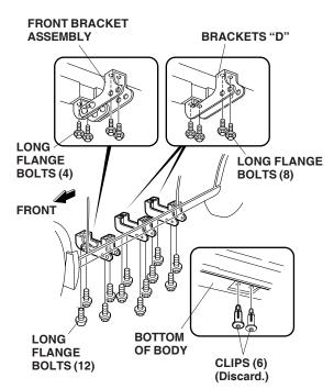
4. On the left side of the vehicle, install the one front bracket assembly and two brackets "D" to the body using the twelve long flange bolts. Thread the long flange bolts in about 3 or 4 threads.
