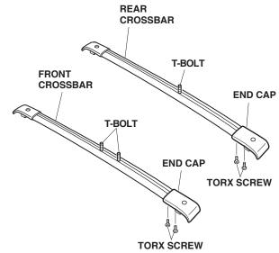
14. *EX model only:* Install the crossbars onto the roof rack, and install but do not tighten the four T-30 Torx screws.
