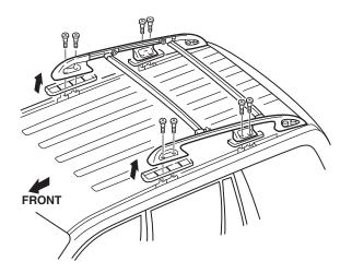
9. *LX model only:* Loosen the knobs on the crossbars, and slide the crossbars off of the roof rack.
