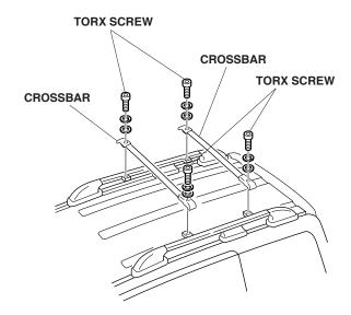
15. *LX model only:* Install the end caps onto the crossbar, and tighten the screws using a T-25 Torx driver
