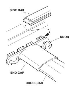
17. *LX model only:* Reinstall the end caps onto the roof rack. Secure the end caps and roof rack with Torx and Phillips screws.
