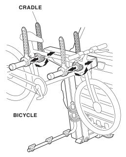
When loading two bicycles, alternate the direction of the bicycles.
