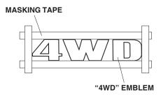
23. Remove the original rear emblem by cutting the outer edges with a piece of string.
