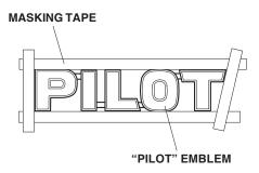
17. Remove the original rear emblem by cutting the outer edges with a piece of string.
