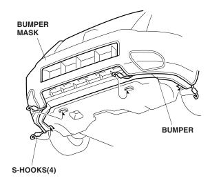
13. Attach the four hooks to the bottom edges of the bumper grille.
