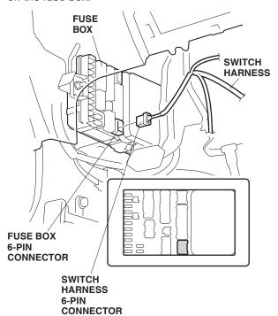
30. Route the switch harness 2-pin connector along the vehicle harness near the parking brake bracket, and locate the 2-pin connector bluetaped to the vehicle harness near the front bulkhead. Remove the blue tape and plug the switch harness 2-pin connector into the vehicle harness 2-pin connector.
