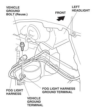
8. Route the short end of the fog light harness 2-pin connector under the left headlight. Locate the 1-pin connector blue-taped to the vehicle harness under the left headlight. Remove the blue tape to free the connector. Plug the vehicle 1-pin connector into the fog light harness 1-pin connector.
