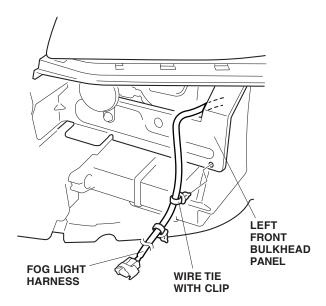
11. Route the fog light harness alongside the vehicle harness and above the fan shroud toward the right (passenger's) side of the vehicle.
