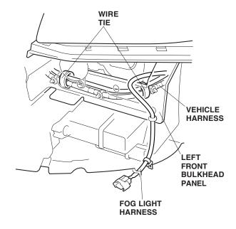
15. Above the left fan shroud, secure the fog light harness to the vehicle harness with two wire ties.
