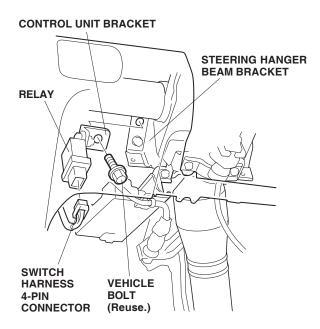
33. Remove the vehicle bolt that secures the steering hanger beam bracket, and attach the control unit bracket with this bolt.
