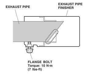
Start the engine and rev it up a few times. Listen for vibration from the exhaust pipe finishers and adjust if necessary.
