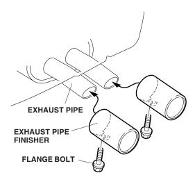
With the flange bolts facing down, slide the exhaust pipe finishers onto the exhaust pipes until they bottom. If necessary, use a rubber mallet to tap the exhaust pipe finishers into place.
