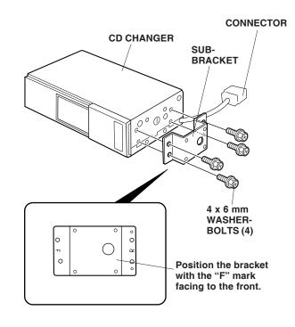
17. Install one CD changer bracket to the connector side of the CD changer with four 4 X 8 mm washer-screws. Attach two wire clips to the lower washer-screws. Install the changer bracket to other of the CD changer with four 4 x 8 mm washer-screws.
