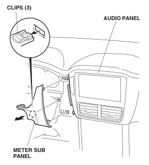
Gently pull out on the left side of the audio panel to release the remaining three clips. Unplug the vehicle connectors and remove the audio panel.
