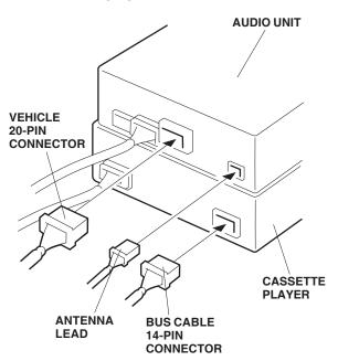
23. Slide the audio unit into the dashboard opening, and reinstall the four screws.
