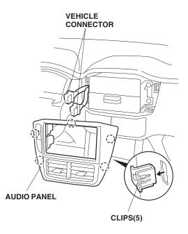
Remove the four screws that fasten the audio unit brackets. Pull the audio unit out toward you, ther unplug the vehicle connectors and vehicle antenna connector from the rear of the audio unit.
