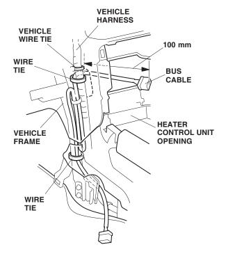
8. Using scissors, cut one EPT sealer in half. Under the driver's center console area, clean the vehicle frame where the EPT sealer will attach. Attach 1/2 of a cushion tape to the vehicle frame at the location shown.
