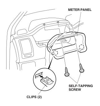
• Remove the meter sub panel (three clips).
