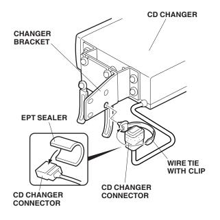
19. Bundle up the CD changer cable and secure it with the two wire clips installed in step 17.
