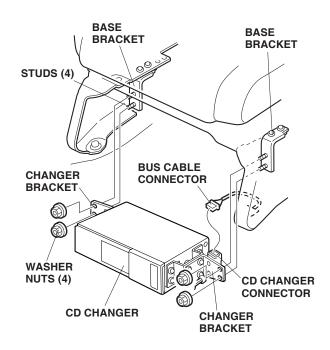
21. Insert the canger brackets over the base bracket studs, and install the one washer nut on the end of each stud. Tighten the washer nuts securely.
