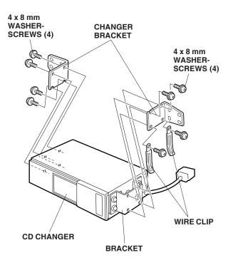
18. Wrap one EPT sealer around the CD changer connector and secure the CD changer connector to the changer bracket with one wire tie with clip.
