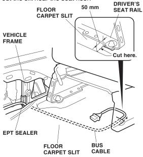
Using the isopropyl alcohol on a shop towel, clean the area where the EPT sealer will attach. Attach half of an EPT sealer to the edge of the vehicle frame in the area shown. 12. Using diagonal cutters, cut and remove the wire tie with clip that secures the vehicle harness to the driver's seat raiser on the center console side.Take care not to damage the vehicle harness when cutting the wire tie.
