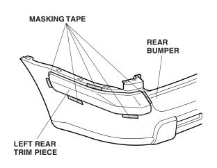
22. Attach a strip of masking tape to the ends of the adhesive backings shown and peel back 2 to 3 inches from the ends. Fold the ends up and tape them to the front of the trim piece. Remove the remaining adhesive backing.
