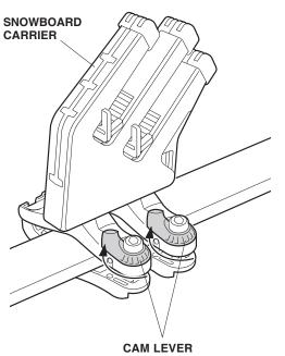
CAM LEVER Return to the original locations. 10. To prevent theft, install the screws in the holes in the top clamps using a TORX wrench.
