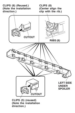
4. Remove the old seals from the 13 clips, and install the new seals from the kit.
