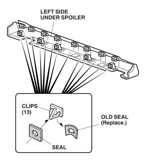
5. Position the left side under spoiler on the body under the front inner fender, and push the clips you just installed into the square holes in the body. Use the palm of your hand to click all 13 clips into place.
