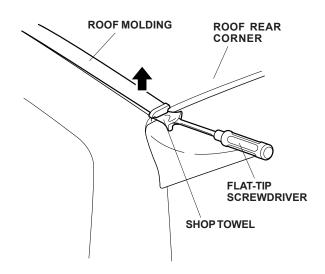
2. Remove the roof moldings by carefully lifting them upward.
