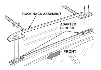
4. Using a T-25 TORX driver, remove the TORX screw from each roof rack crossbar (front and rear) on one side of the roof rack, then remove the side rail from the roof rack.
