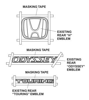
7. Remove the "H", "ODYSSEY" and "TOURING" emblems from the body by cutting the outer edges with a piece of string.
