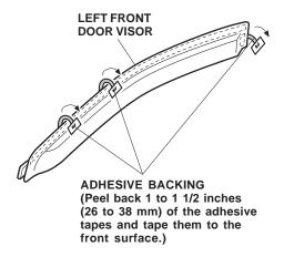
Position the left front door visor on the door. Push the front retaining bracket into the door mirror base; push the two rear retaining brackets into the door sash.
