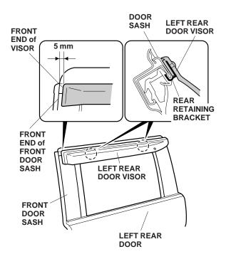
12. Adjust the visor so that the clearance between the front end of the visor and front end of the front door sash is 0.2 inch. (5 mm).
