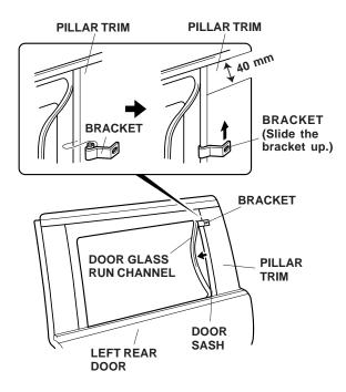
Position the left rear door visor on the door sash.
