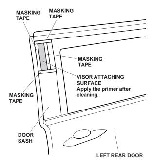
9. On the back of the left rear door visor, peel back 1 to 1 1/2 inches (26 to 38 mm) of the adhesive backing, and tape the backing to the front surface of the left rear door visor.
