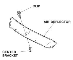
7. Pull down on the rubber molding from the inside edge of the hood, and slide the two front brackets and two side brackets over the lip of the hood, under the rubber molding. Align the holes in the brackets with the holes in the plastic grommets, and install one truss screw through each bracket.
