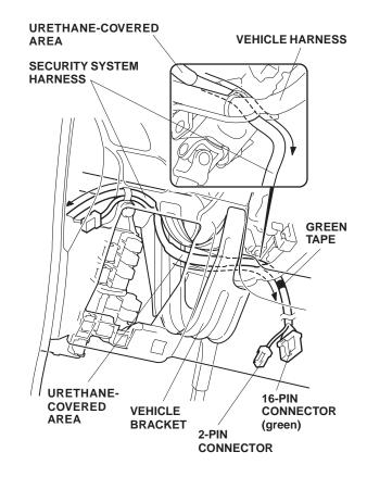
8. Attach the clip band in the kit to the security system harness at the green tape, then push the clip into the vehicle panel hole.
