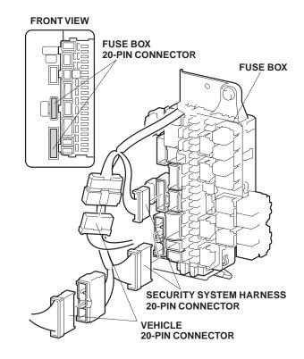
12. Remove the dummy connector from the keyless entry harness.
