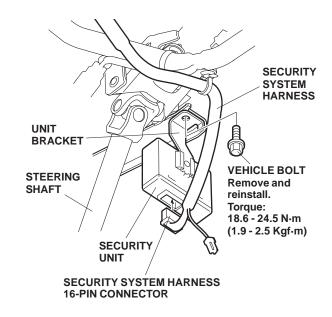
18. Plug the security system harness 16-pin connector into the security unit.
