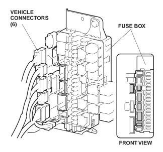
11. Plug the security system harness 20-pin connectors in between the fuse box 20-pin connectors.
