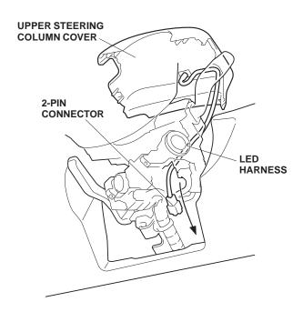
25. Secure the LED harness to the vehicle harness using three wire ties.
