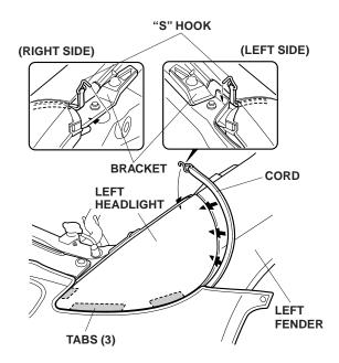
Pull the mask back toward the wheelwell, smooth out any wrinkles, and snap the mask to the snapscrew. Attach the three plastic hooks to the fenderwell.
