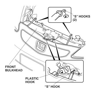
11. Attach the four hooks to the grille opening. Insert the two tabs between the grille and the front bumper, and attach the four plastic hooks to the bottom edges of the front grille.
