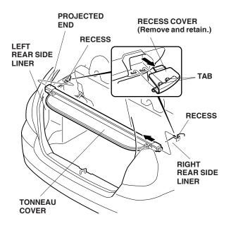
2. Insert the left end of the tonneau cover into the recess in the left rear side lining, then compress the tonneau cover and insert the right end into the recess in the right rear side lining into position, until set right end clicks.
