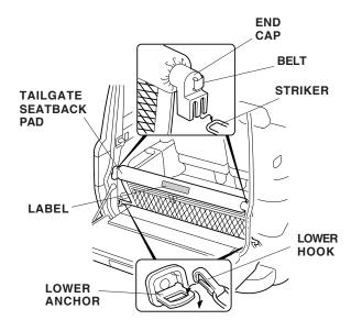
2. Attach the tailgate seat back pad lower hooks to the left and right lower anchors on the vehicle.
