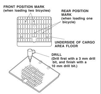
5. Using a utility knife, cut out the foam blocks from the underside of the cargo area, as shown.
