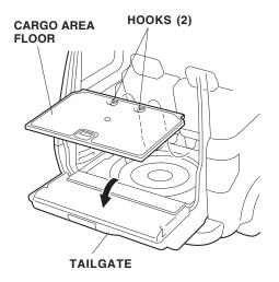
Turn the cargo area floor over, and locate the four marks on the underside of the cargo area floor.
