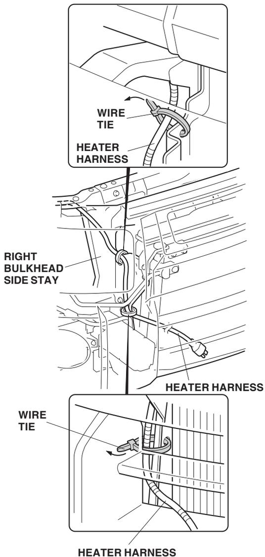
13. If you are also installing fog lights, secure the heater harness to the fog light harness with two wire ties as shown. If the vehicle you are working on is equipped with A/C, check that the heater harness is not interfering with the A/C pipes.
