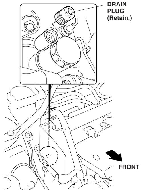
6. Install the engine block heater with the aluminum washer into the bolt hole using a 24 mm socket and a torque wrench. Torque the engine block heater to 60 N·m (44 lbf·ft).
