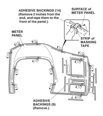
3. Position the meter panel on the existing meter panel. While holding pressure on the meter panel, carefully remove the adhesive backings from the meter panel. Press the meter panel firmly against the existing meter panel with the palm of your hand, particularly at the edges.
