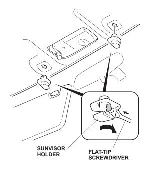
5. Remove the cap from the left sunvisor (four retaining tabs).
