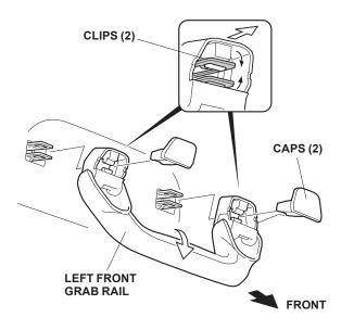
15. Using a flat-tip screwdriver, remove the grab rail from its two clips.
