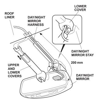
26. Slide the upper cover up under the roof liner.
