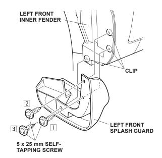
Turn the steering wheel all the way clockwise, and repeat steps 2 and 3 to install the right front splash guard.
