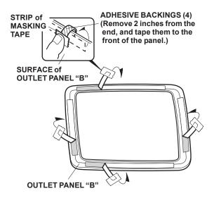
10. Position the outlet panels "A" and "B" on the existing outlet panels. While holding pressure on the outlet panels, carefully remove the adhesive backings from the outlet panels. Press the outlet panels "A" and "B" firmly against the existing outlet panels with the palm of your hand, particularly at the edges.
