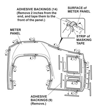
Position the meter panel on the existing meter panel. While holding pressure on the meter panel, carefully remove the adhesive backings from the meter panel. Press the meter panel firmly against the existing meter panel with the palm of your hand, particularly at the edges.
