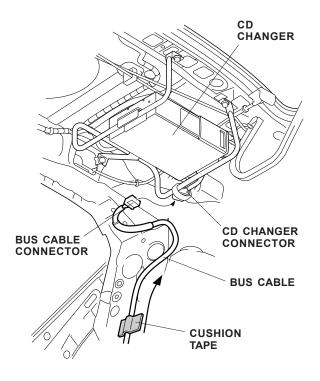
38. Fold the excess BUS cable, and secure the BUS cable to the holes in the rear seat panel with the two wire ties with clips.
